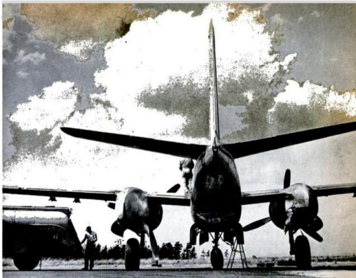
TRICYCLE LANDING GEAR and slender fuselage show up in this rear-end view. Four Douglas-type, double-slotted flaps—two under the wings and two between engine nacelles and fuselage—slow down the "hot" A-26 for landings on short advanced-base fields. Large control surfaces boost maneuverability.
