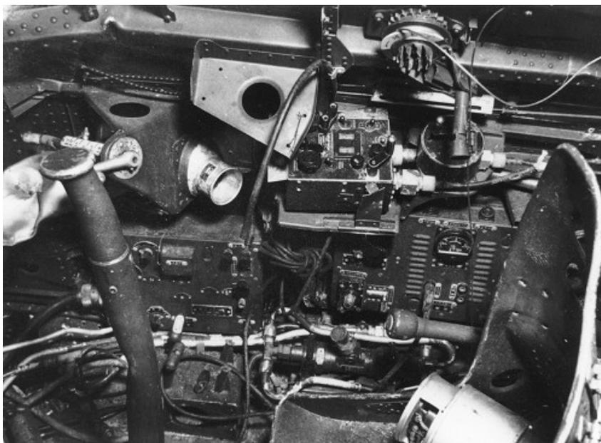
**Interior view of the Zero cockpit which crashed into Building 52 at Fort Kamehameha, note the U.S. manufactured Fairchild Radio Compass in the upper center (Compass Model RC-4, Serial # 484). It was tuned in on 760 KC, official US Navy photograph**
