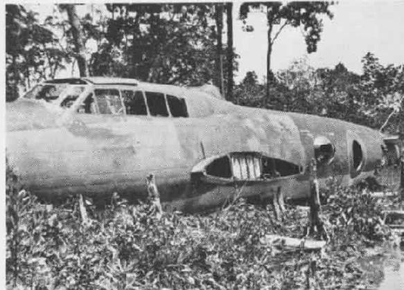
**3** With wings and tail surfaces removed, fuselage of *Betty* lies in swamp, ready for the big job of moving it to tidewater for re-shipment; *Betty* is Japan's fastest bomber, carrying five to seven men at speeds up to 288 mph, flying as high as 29,000 ft.
